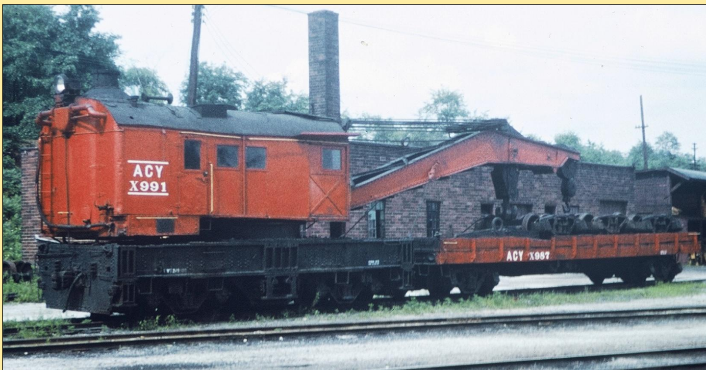
Above: AC&Y's relief wreck derrick X-991 was photographed at Brittain yard with boom idler car X-987 in May 1957 about four years after it was refurbished. Originally in bright red attire, AC&Y's X-991 was repainted blue shortly after the AC&Y merger into the N&W System in 1964. Ed Kirstatter.
