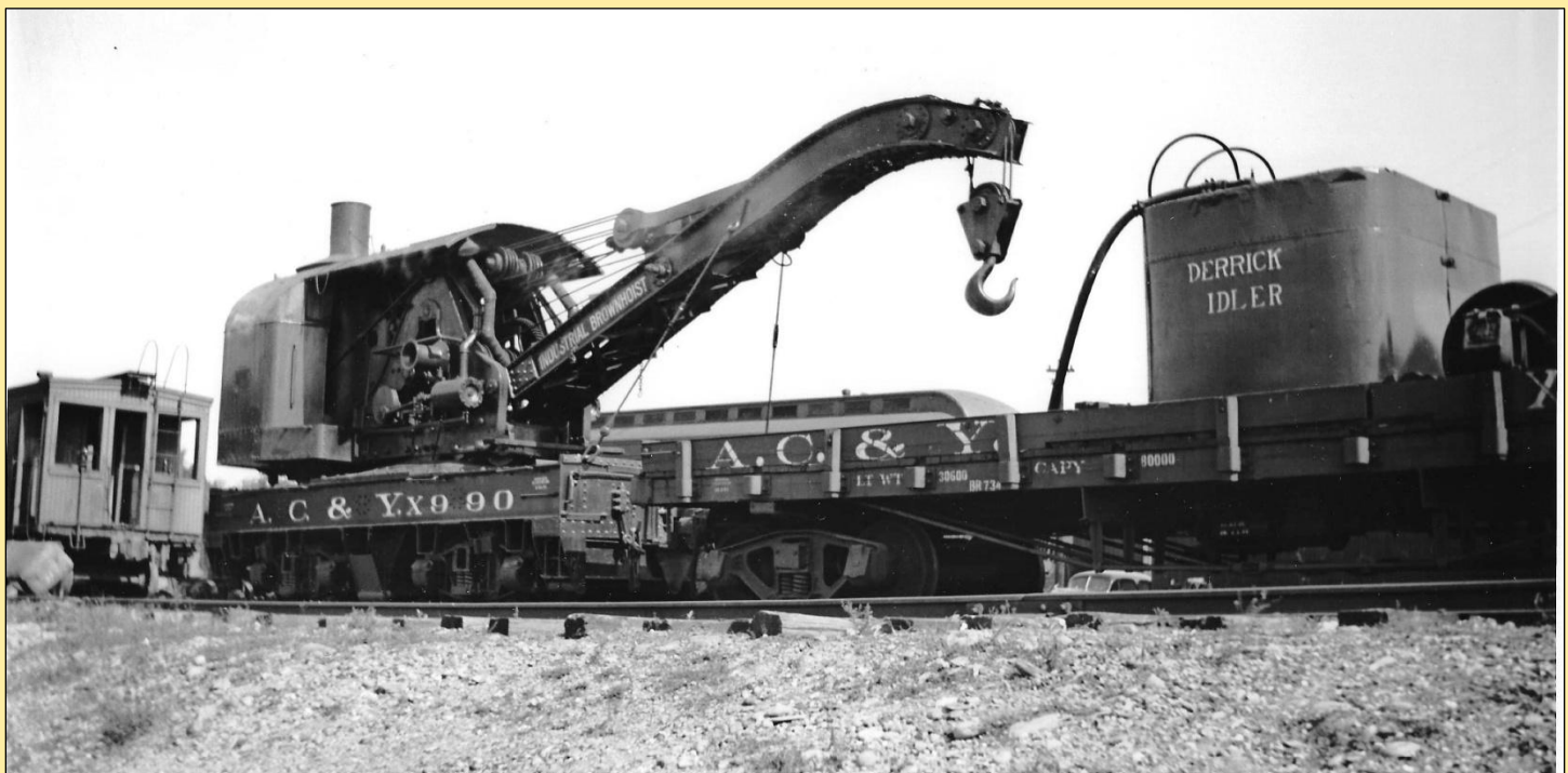
Above: Repainted steam wreck derrick X-990 and idler X-985 (first X-985) are seen at Brittain yard in September 1935. The 50-ton derrick is believed to be painted black with a red (lead) roof. Jay Williams collection.
