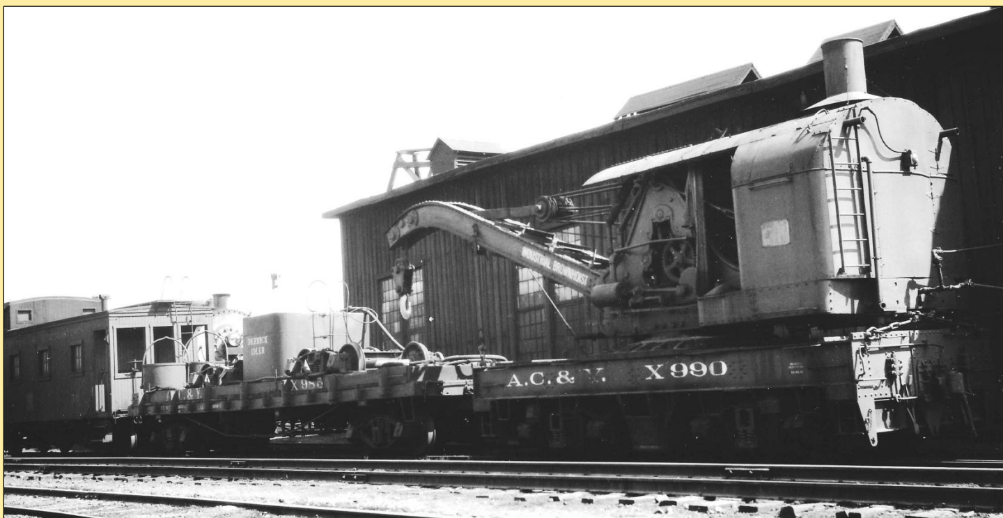
Above: AC&Y's X-990 steam derrick and idler X-985 (first X-985) are held on the Brittain Stores track in 1935 with caboose 50. The piping leading from the roundhouse boiler to X-990 provided a ready source of preheated water in case the wreck outfit was needed for emergency clean-ups or right-of-way work train assignments. Jay Williams collection.
