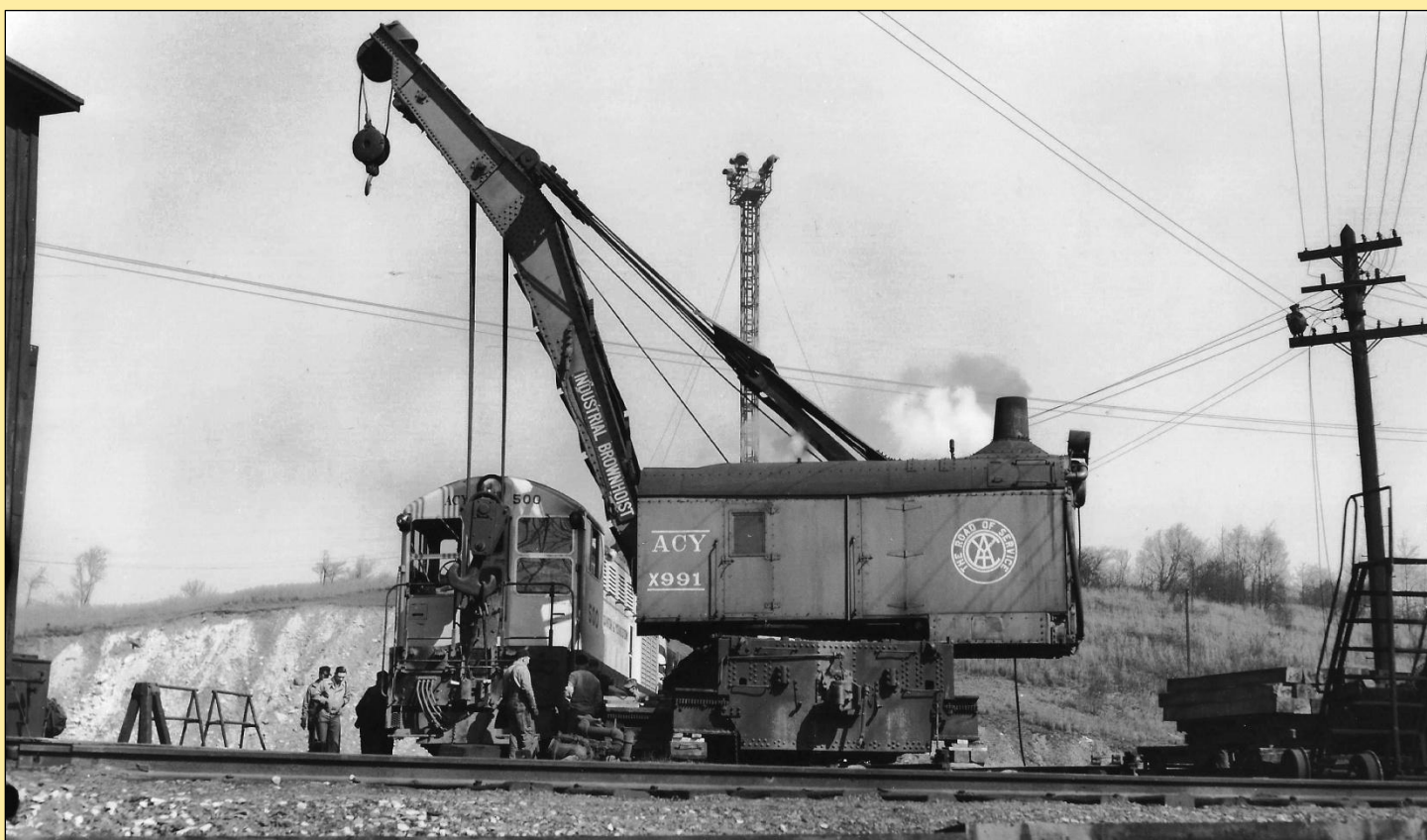
Above: AC&Y's wreck derrick X-991 was purchased May 1935 and retired September 1973. It was always steam powered as seen in this undated photo sometime after 1948. Under AC&Y's dieselization program, a new oil fired burner was installed in June 1953, replacing the coal fired boiler. The X-991 was often utilized for work assignments beyond derailment clean-ups. Bob Richardson, courtesy DeGolyer Library – SMU – Dallas, Texas.
