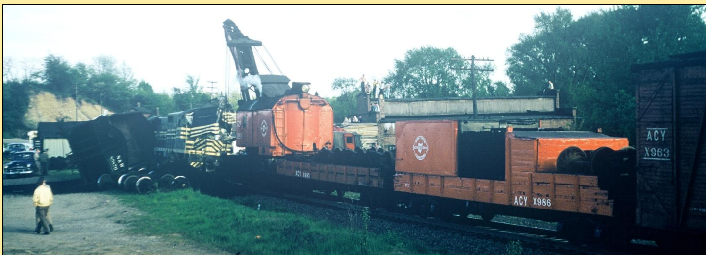
Above: The AC&Y wreck outfit is working a rear-on collision involving NKP GP-7 447 and a 700-series caboose in June 1956 on the NKP at Mogadore. The X-991 derrick is now oil fired. Ed Beckwith, Chris Lantz collection.
