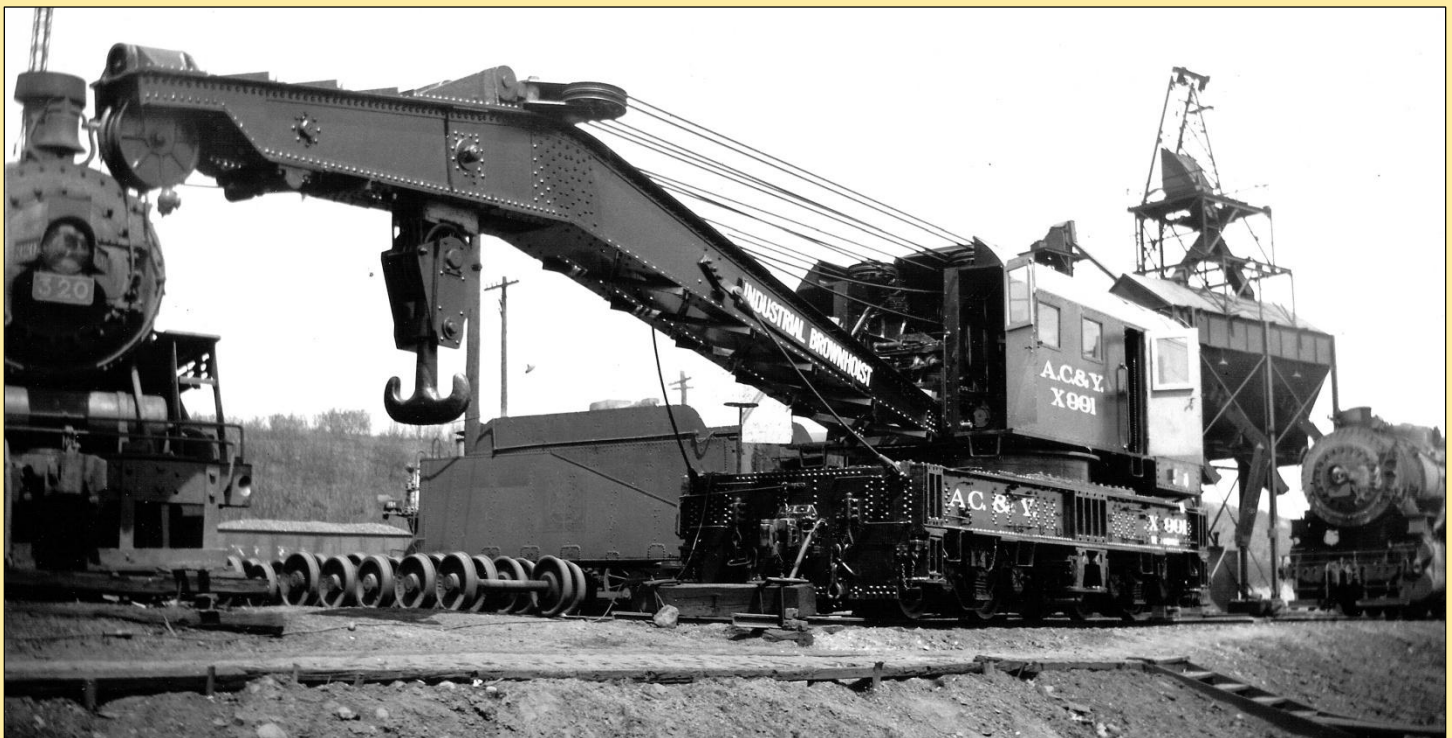
Above: On display at Brittain yard in 1935 is the AC&Y's newly arrived 160-ton capacity relief wreck derrick X-991. Note the fresh paint and light colored roof, either white or aluminum gray. Typically, AC&Y's relief roster was later bright red with gloss black paint applied to the frame, underbody and trucks. The boom proudly proclaims the manufacturer, Industrial Brownhoist Company of Bay City, Michigan. Bruce Triplett, Bob Lucas collection.
