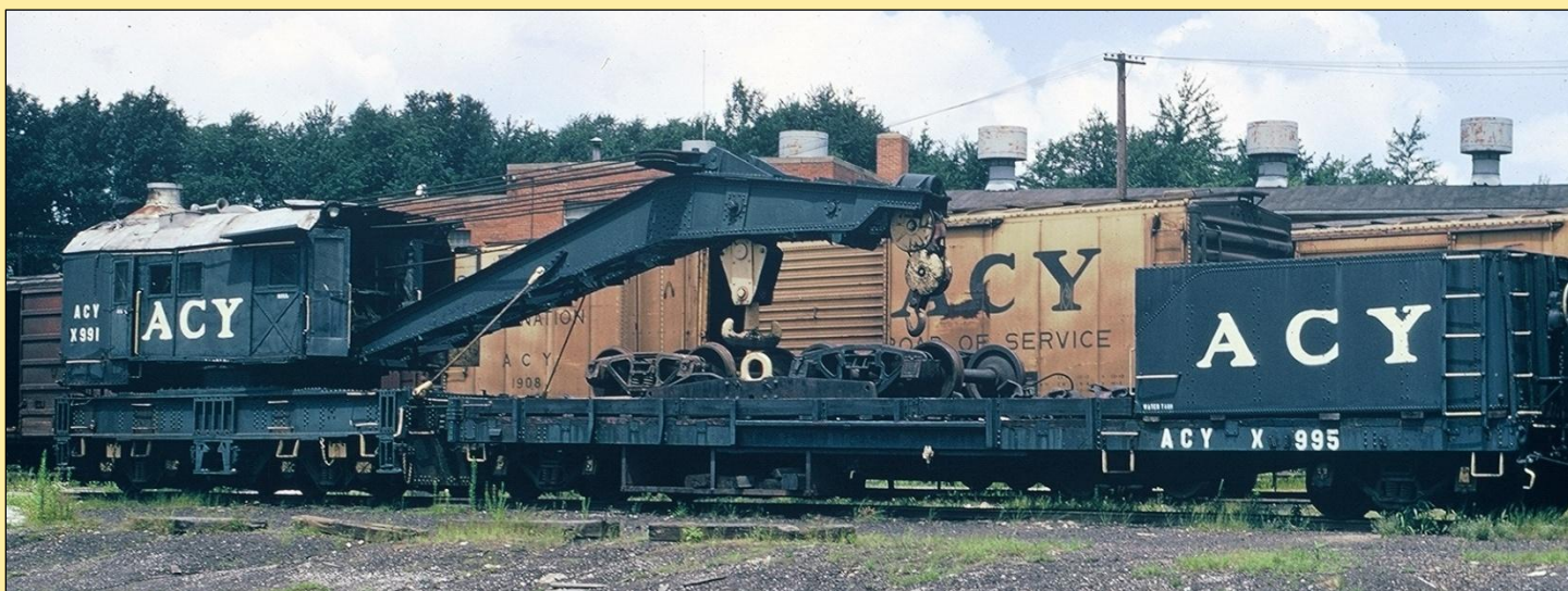
Above: Good images of AC&Y derrick idler X-995 are surprising rare. Converted from leased 50' boxcar 3809 in November 1968, the X-995 was retired in September 1973 after less than five years service. It appears the water tank was salvaged from tie-rail-water car X-986. Michael Bradley collection.
