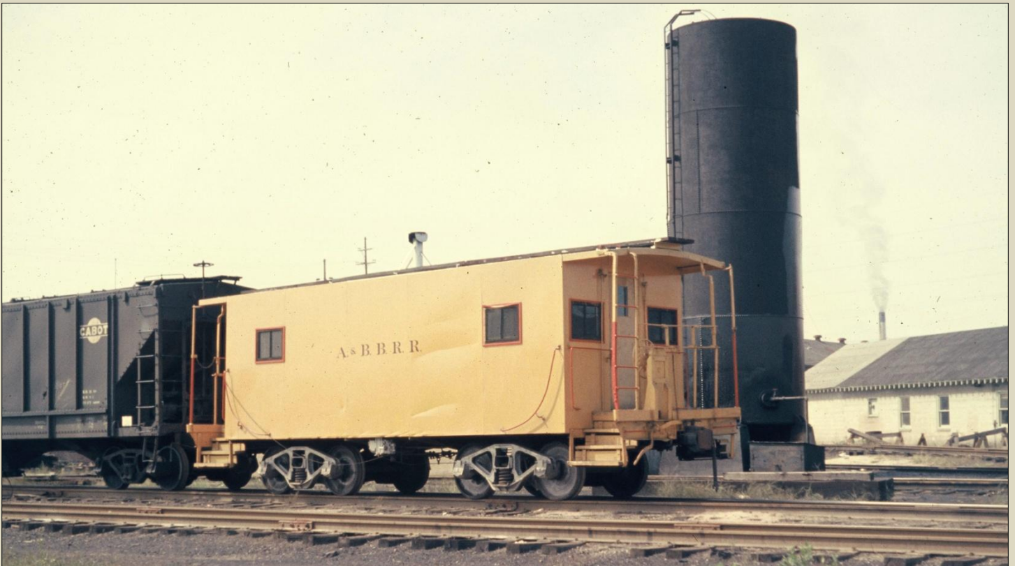
ABOVE: Clearly well maintained and recently repainted, A&BB caboose 2 appears about 1962 at Barberton, most likely returning from an East Akron transfer run. Long thought to be plywood construction, personal accounts of A&BB trainman confirm caboose 2 was steel sheathed. (John Beach)
