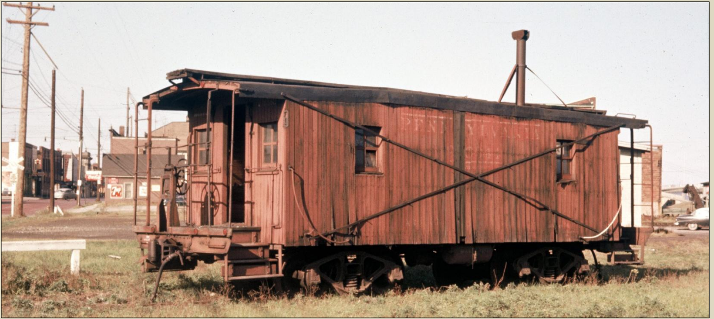
ABOVE: At Barberton about 1963 is the derelict A&BB caboose 1. The car also was an ex-Pennsy class N6B cabin number 983044 that came to the Belt Line in January, 1947. It apparently had structural issues at some point, serious enough that the A&BB backshop installed tie rods to keep the car squared up. Notice the Pennsylvania road name and number are still discernable behind the faded red paint. (John Beach)
