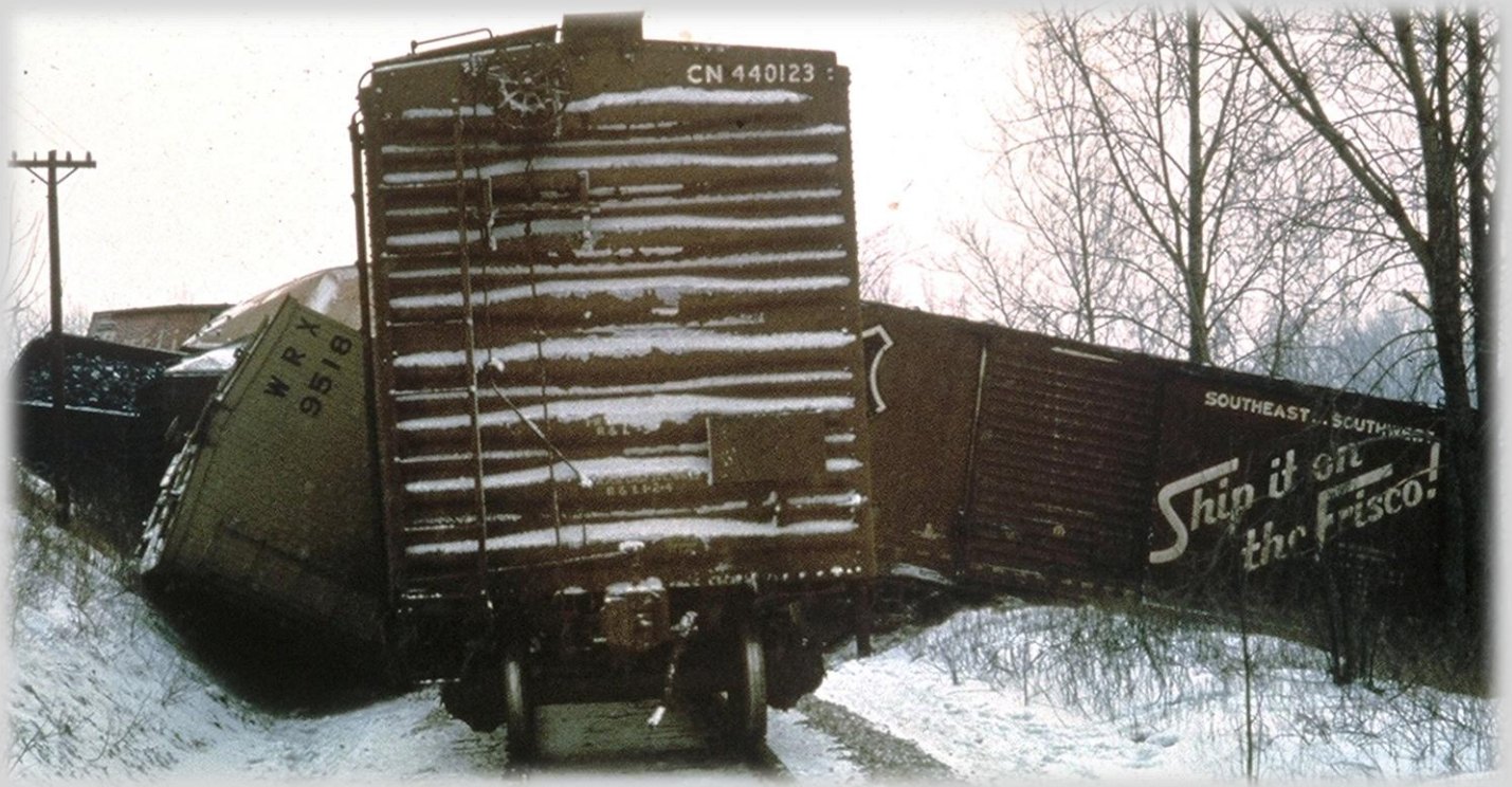
Above: Nearly all of the freight cars involved in the derailment were Post-War modern steel construction. Yet, one vintage car appears behind the CN box. WRX No. 9518, a 40-ton ice-bunker refrigerator, was one of a small number of cars owned by the Western Refrigerator Line for the Green Bay & Western Railroad. This car was built between 1932 and 1936. Jim Roberts' photo, author's collection.
