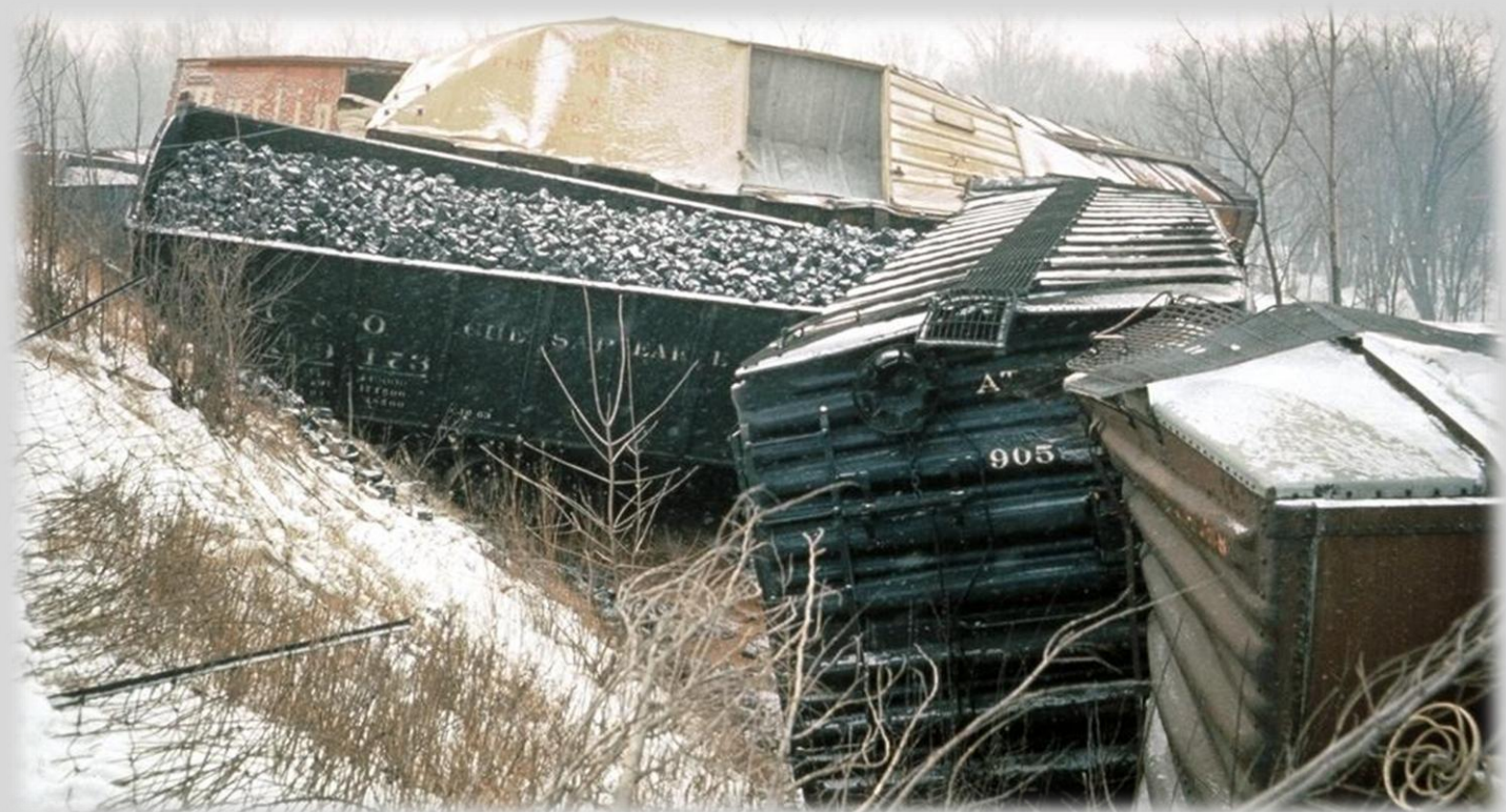
Above: Looking southeast are “dominoed” freight cars. The C&O hopper with coke for the Ford Motor Cleveland Foundry was a total loss. The Santa Fe box contained crude rubber destined New Jersey. The load was transferred. The car was home-shopped. Eighteen of 27 cars involved were destroyed. Jim Roberts’ photo, author’s collection.
